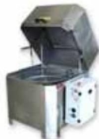
Degreasing and cleaning of parts in basket washers with translational or rotational mechanical movement.
