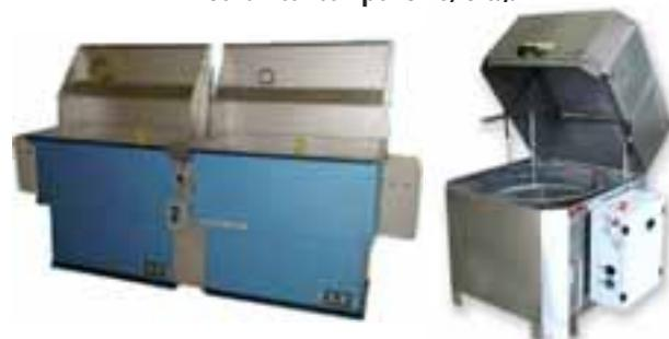
NEUTRALÈNE® BIO 1000 can be used in cold or hot tanks up to 158 °F and in rotating or forward-travelling basket machines.
