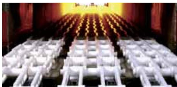
Industrial oven chain conveyor lubrication. Continuous firing of phenolic/silver conductive polymers at 428 °F
