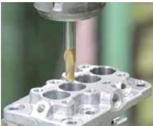
Center point drilling on light aluminium-silicon alloys,
