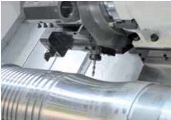
Pilot hole drilling with classic drill chuck and bits
