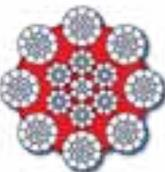
Internal lubrication can be provided by the manufacturer. Contrary to accepted ideas, internal lubricants are compatible with external lubricants most of the time.
